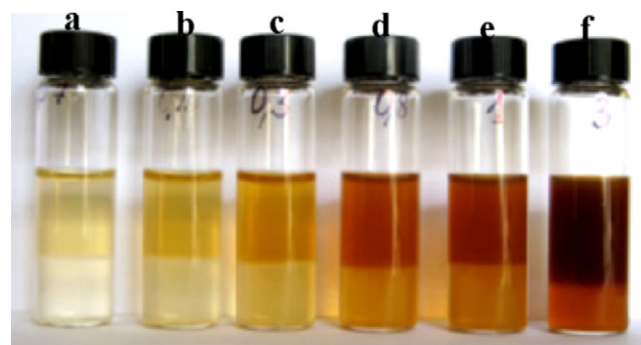
Fig. 3. Photos of swollen microgels (sedimented) at equilibrium in the excess of PVP/C60-1.2 aqueous solutions of 0.07 (a), 0.1 (b) 0.3 (c), 0.8 (d), 1 (e) and 3 (f) g/dL.
